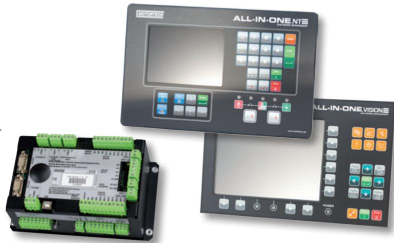
AIO supports many standard ECU (electronic control unit) types and is specially designed to easily integrate new ones. A powerful graphic display with user-friendly controls allows any user whatever their ability to find the information they need. The display on the basic version is capable of displaying graphical languages (e.g. Chinese).
